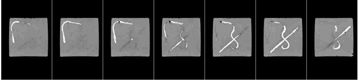
Figure 2.6: Selected slices of the T_1 -weighted image of the rat phantom showing the phantom configuration. Two of the spinal cords are put together to create a fiber crossing region.
